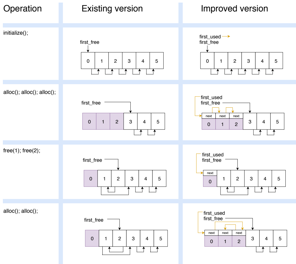
Figure 4.3: Improved static memory block allocator
